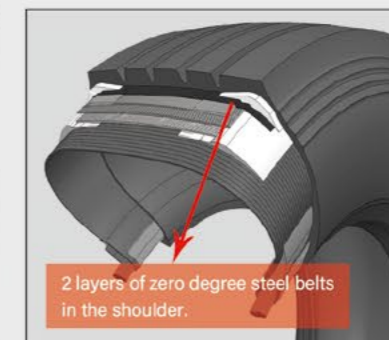
ZERO DEGREE STEEL BELTS STRUCTURE TECHNOLOGY (ZDST) SIDEWALL: 1 STEEL LAYER TREAD: 4 STEEL LAYER
